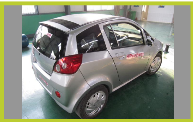
Hirate Energy's own EV prototype, consisting of an 11kW SRM motor and controller system, a 120V120Ah gel battery pack, and an active BMS.
